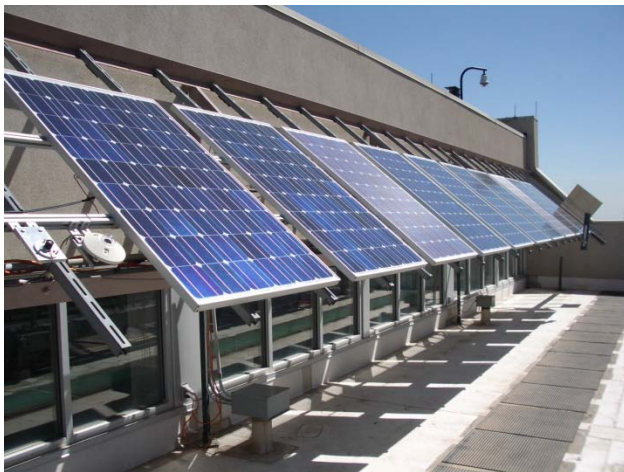
Fig. 2: Mounted solar modules and pyranometers. Shade obstructions for Test #2 are visible at the far right.
